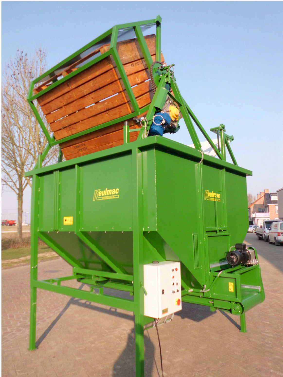
2.50 x 2.50 meter version with electric tipper
