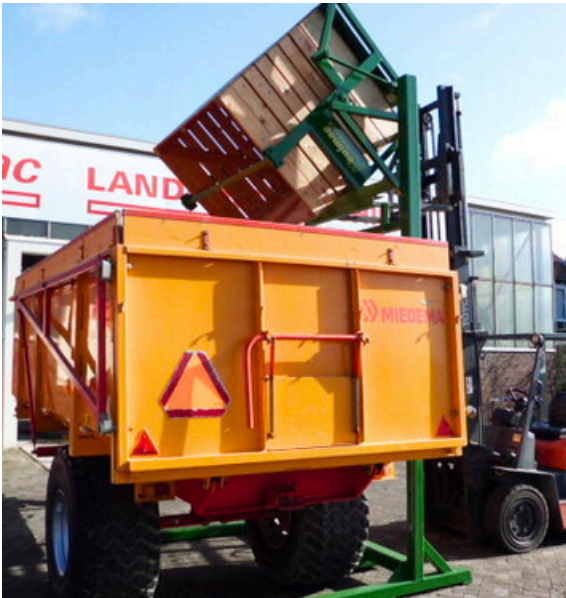
mechanical box tipper tilted with the forklift truck
