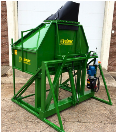
hydraulic box tipper with elektr./hydr. unit, optional: cover plate with rubber outlet
