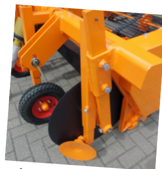
double convex disc left side
